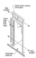
Is the opening the correct size for the door unit? Check it against the door frame size now, before installation. The opening should be frame height plus 1/2 inch, and frame width plus 1/2 inch.
