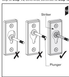
13. The striker allows 2.5mm (3/32") of adjustment in each direction when the striker face plate is fitted in the centre of the striker body.
