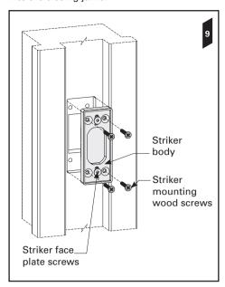
10. Remove the striker face plate screws. The striker nuts are now trapped in position.
