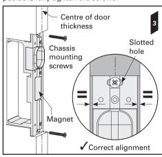
**4.** Fit the 6x side handle to chassis screws. **Leave a 3mm gap** (1/8") between the underside of the screw head and the chassis.
