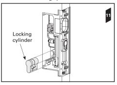
**12**. Secure the locking cylinder using the locking cylinder screw. DO NOT fully tighten the screw.
