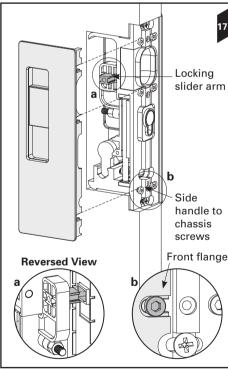
**18.** If installing a 'Key/Key' handle you may need to adjust the position of the locking cylinder. To do so, insert the locking cylinder Allen key through the slotted hole in the chassis. Loosen the screw and slide the cylinder into the desired position. Tighten the screw.
