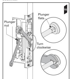
**16**. Continue to turn the spanner until there is no longer a gap between the spanner and the shroud face.
