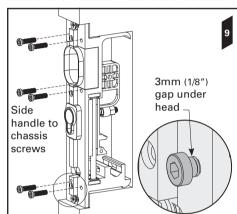
10. Fit the key locking side handle with the keyhole cut out to the chassis by sliding the front flange of the handle under the heads of the 3x side handle to chassis screws. Tighten the screws.
