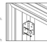
screws. For middle and bottom hinges, proceed to install one (1) #10 x 2-1/2" screw in the bottom hole, closest to the weatherstrip.
