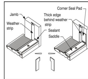
Apply sealant (Polyurethane or Elastomeric) at the joint where the threshold cap meets the jambs and mull posts.
