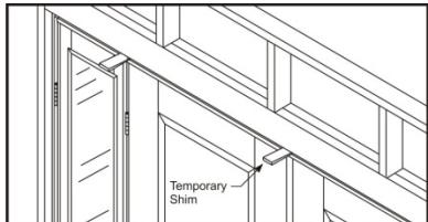
When installing a French door with active sidelites, place temporary shims above the center of the head frame, where doors meet. Pre-drill and insert a screw through frame into header, then remove the temporary shims.
