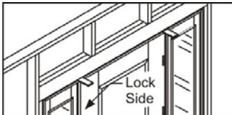
Shim directly over lock side mull post. Recheck lock mull post to ensure weatherstrip contact is even top to bottom. Finish driving screw tight.
