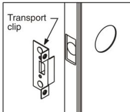
Remove transport clips. Confirm door and sidelites operate properly.
