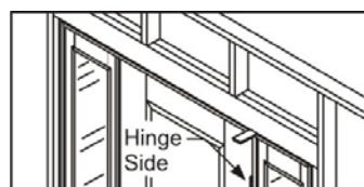
Shim directly over hinge side mull post. Using a 6 foot level, recheck hinge mull post to ensure it is plumb and straight. Finish driving screw tight.
