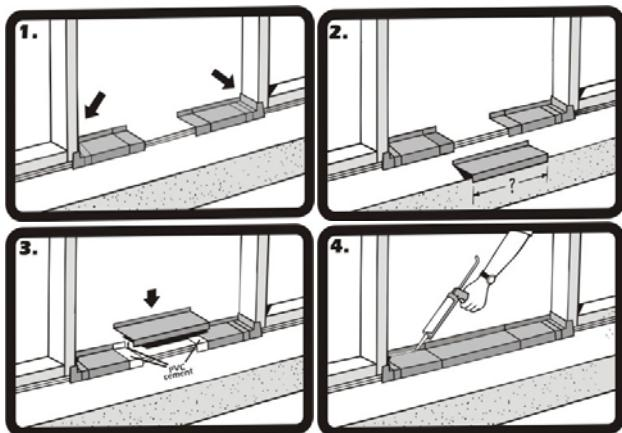
**Note:** Use only the PVC cement provided in the sill pan kit to glue the pieces together. The sill pan must be sealed to the sub-floor using an Elastomeric or Polyurethane sealant, but do not apply sealant to the bottom of the sill when using a sill pan.
