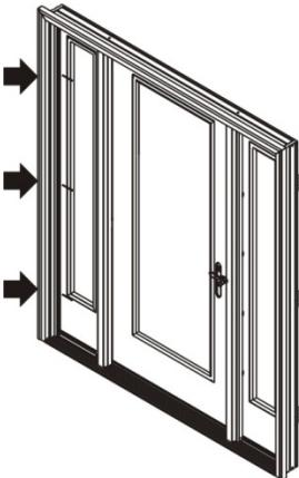
Adjust the sidelite hinge jamb on the hinge mull side of the unit to obtain even weatherstrip contact top to bottom at the lock side of the sidelite. Place a screw through the hinge side jamb, into the stud, at each remaining hinge location.
