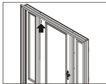
Use a 6 foot level and plumb the hinge side mullion both ways (right to left and inside to outside).
