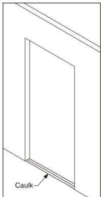
On the sub floor at opening, place 3 very large beads of sealant. Run beads full width of the opening.
