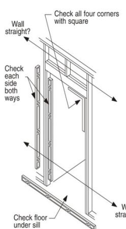
Is the opening the correct size for the door unit? Check it against the door frame size now, before installation. The opening should be frame height plus  $\frac{1}{2}$  inch, and frame width plus  $\frac{1}{2}$  inch to  $\frac{3}{4}$  inch. **Fix any problems now.**
