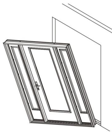
Lift the unit up. With top edge tilted away from opening, center the unit and place sill down onto sill pan or caulk beads and tilt into opening. For all door unit configurations, note the hinge locations and mark those locations on the jamb faces near the door surfaces. Pre-drill 1/8 inch diameter holes at these locations and through the head jamb adjacent to the mullions, over the active sidelites. A counter sink bit will help to conceal the screw heads.
