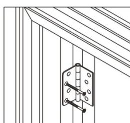
With sidelites open, drill 1/8" diameter pilot holes and install the long hinge screws in the hinge locations closest to the weatherstrip. Do this for all hinges.
