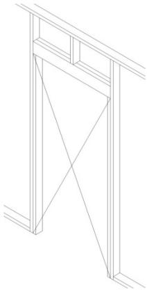
Check to be sure the framing walls around the opening are in the same plane. Do this by performing a "string test" for plumb.
