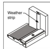
After adjusting the threshold cap, ensure that the weatherstrip is **flush** with the top of the threshold cap. Trim as necessary.
