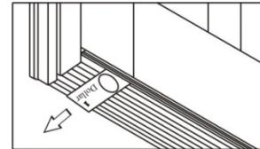
This check should be performed at each adjustment screw location on each active threshold cap.
