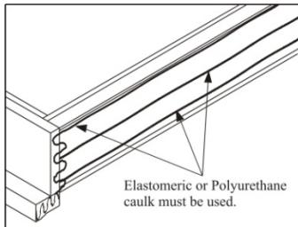
Lay the door unit on edge or face so that the bottom surface of the sill can be caulked. Place very large beads of caulk across the full width of the sill. Additionally, place beads of caulk along the junction of the sill and the jamb and on the bottom surface of the jambs and brickmould.
