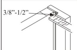
Adjust lock side mull post so that the weatherstrip contacts the door surface equally at the top, middle, and bottom, an even 3/8" - 1/2" when fully closed. Place a screw through the pre-drilled hole in the head jamb at the lock side mullion.
