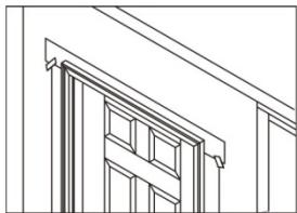
Provide and maintain a properly installed drip cap or head flashing to protect top of surfaces from **Water intrusion** and damage. Tape and properly seal the top flap of the Water Resistive Barrier (WRB) over the head flashing.
